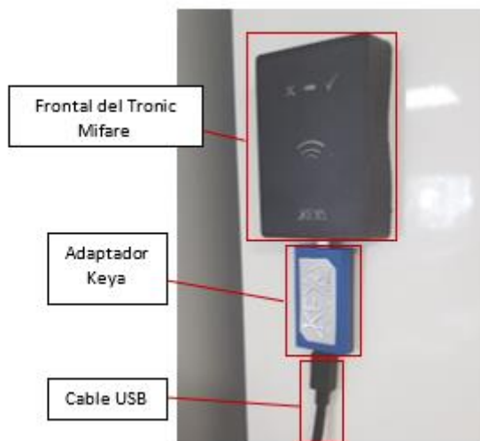
Figure 3: Connection of the cables to the lock
