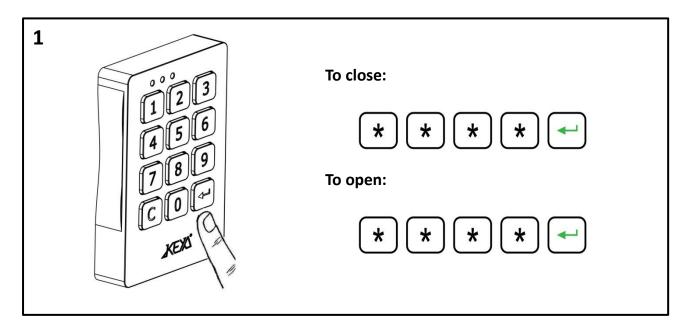
Open and close by 4-digit code. The code is erased every time the lock is opened, being available for a new use.
